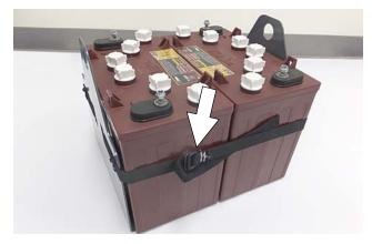
6. Using an approved lift strap that supports the weight of battery pack, connect the strap to the two lift brackets as shown. Using a lift hoist rated to handle the weight of the battery pack, carefully lift the battery packs to and from machine. Keep one hand on the battery lift box when lifting for stability.
